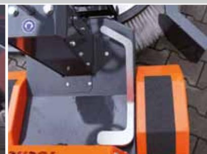
Ergonomically shaped foot pedal for the traction drive
