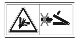
Do not touch any moving machine parts. Wait until they have come to a complete standstill.
