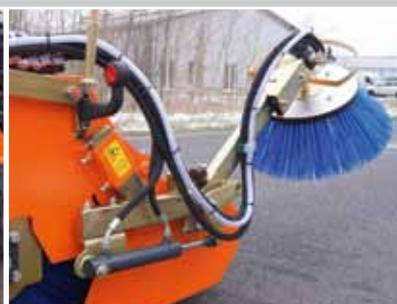
Hydraulic side brush w/hydraulic lifting and lowering
