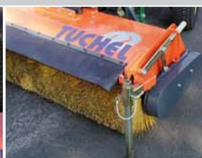
Adjusting-lever and parking stand
