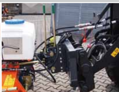
Yard loader / Front loader attachment with parallelogram
