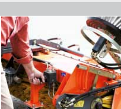
side brush incl. speed adjustment
