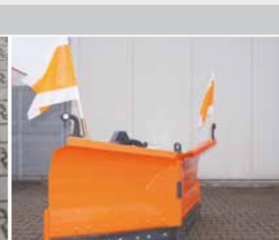
VARIO incl. road traffic equipment (flags and lights)
