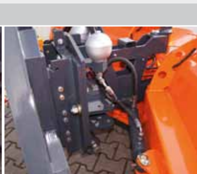
Hydraulic angling of the folding wings
